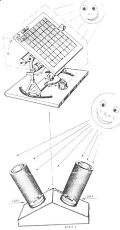
geared motors of the type used for models, with a suitable voltage and maximum operating current of 300 mA, are suitable for driving the solar panels. The use of this control circuit makes it possible to control the solar panel in one plane. Of course, to track the sun from sunrise to sundown, two control circuits will be required: one for horizontal and one for vertical tracking.
