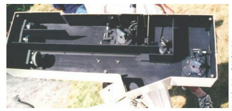
Now onto the instrument. Using this image of the optical layout, notice that there are **two** gratings. The first acts as the input to the prominence scope and is 2" x 2" grating with 1200 lines/mm used in the second order. It is blazed for a wavelength of 500nm in the
